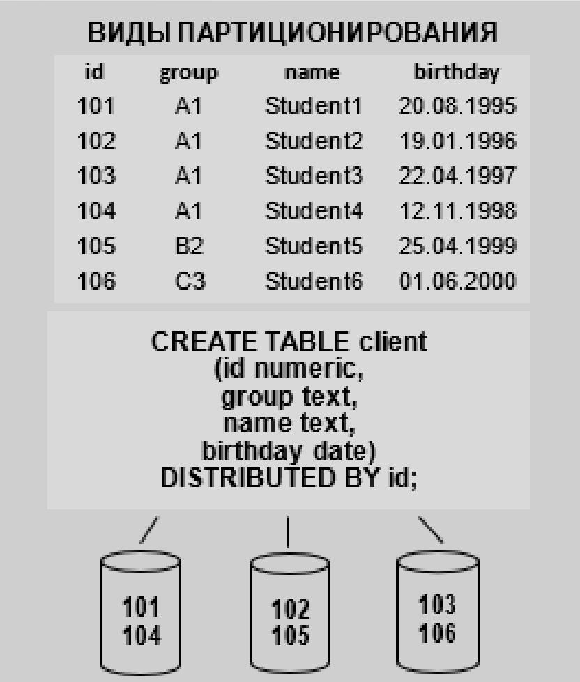
The diagram illustrates the distribution of data across three partitions based on the `id` column. The first partition contains rows 101 and 104. The second partition contains rows 102 and 105. The third partition contains rows 103 and 106.
